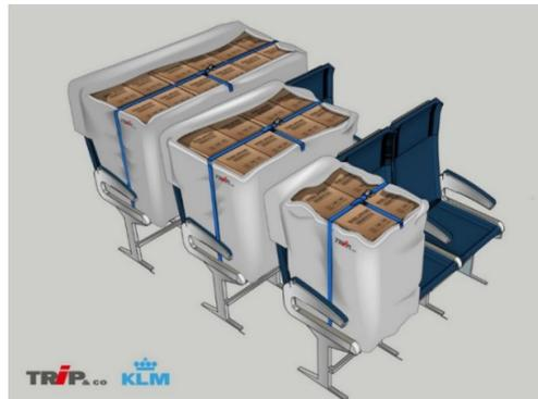
Fig. 5. Example of a CSB with a triple-seat variant
