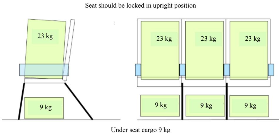
Fig. 3. Interim cargo transportation on seat for three boxes maximum 23 kg
