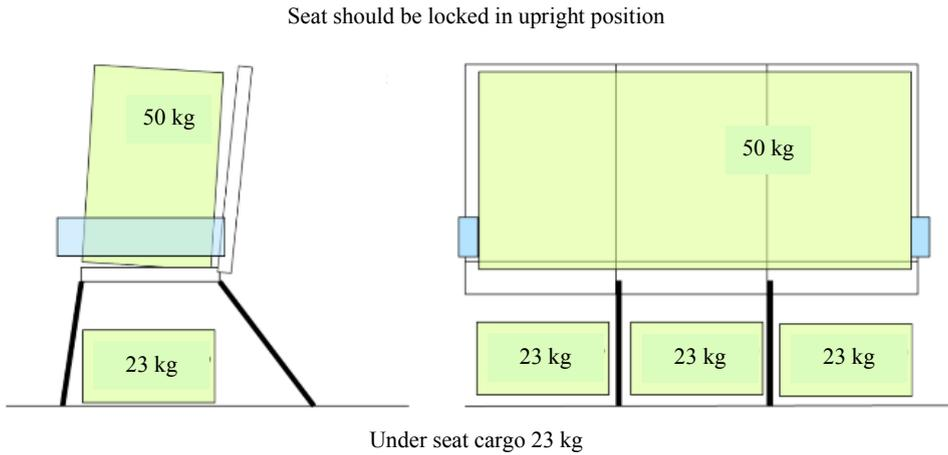
Fig. 4. Interim cargo transportation on seat for one box maximum 50 kg
